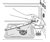
When using water of medium hardness, the regenerating salt container should be refilled after approximately **20 washing cycles**. The salt container can hold approximately **1 Kg** of salt in grains. The container is situated at the bottom of the dishwasher. After removing the lower basket, unscrew the salt container cap by turning it anticlockwise and pour in the salt using the funnel supplied with the dishwasher. Before replacing the cap, remove any salt residues from around the opening.
