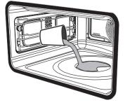
Spray a water and washing up liquid solution inside the oven using a spray nozzle. Direct the spray against the side walls, upwards, downwards and towards the deflector.
